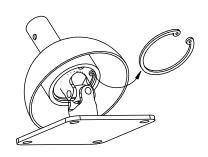
4. Disassemble the Seeger circlip using special pliers.
